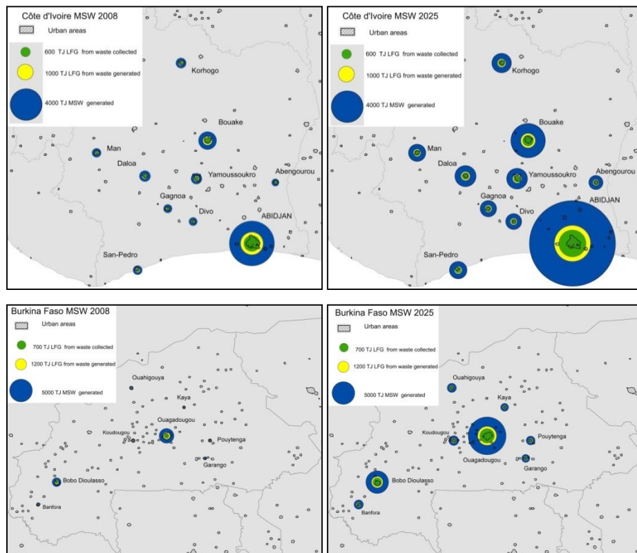
Figure 3. Spatial distribution of energy potential of waste - exemplification for Burkina Faso and Côte d'Ivoire
